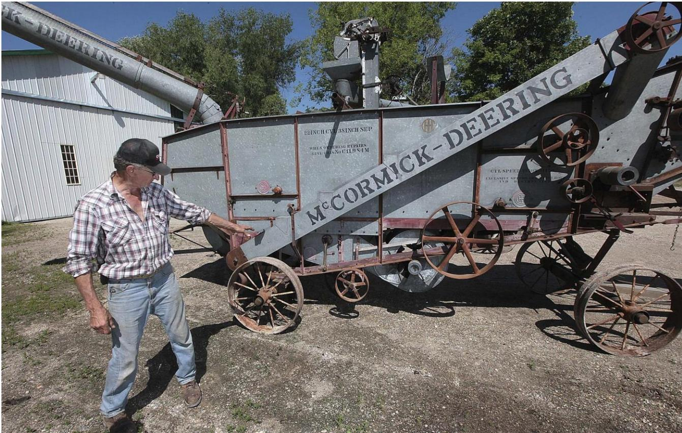
Barry Klym points out the flywheels on his McCormick-Deering 22x38 threshing machine and what it will do when hooked up to a series of drive belts powered by his 1935 tractor.
