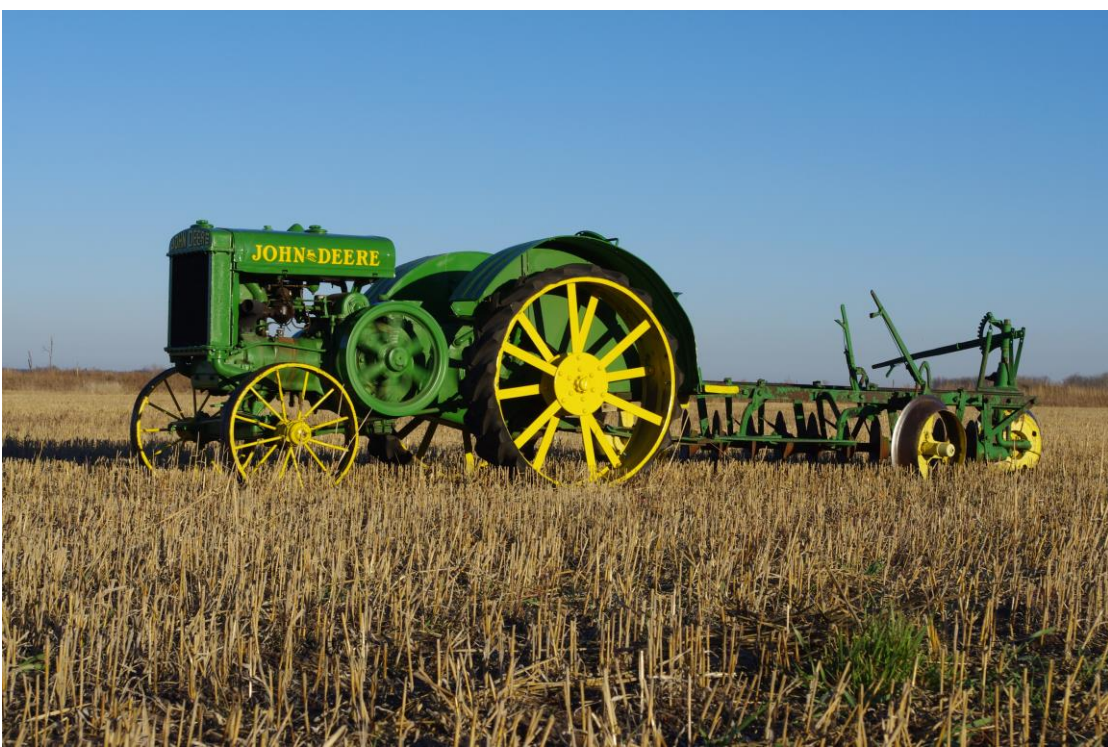
The Museum’s Model D tractor on a sunny fall day. Even through the tractor is running the spoked flywheel can be clearly seen.
