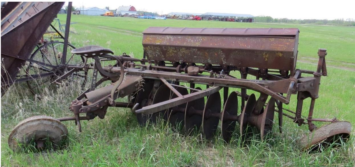
*A four-foot wide Cockshutt tiller combine set up for horse operation with an operator's seat attached to the machine. Oddly enough, this tiller combine features a rubber tire on the front left corner. Whether this tiller combine left the factory with a rubber tire is not known to the Museum. While possible, it is an odd set of options.*
