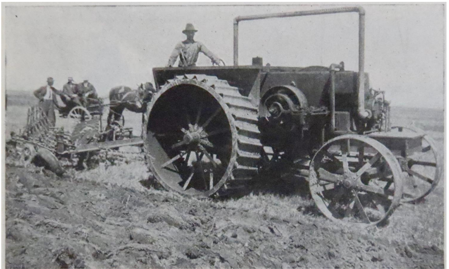
Goold, Shapley & Muir 15-25 "Ideal" Kerosene Tractor, pulling a 5-bottom Cockshutt Powerlift Engine Gang
